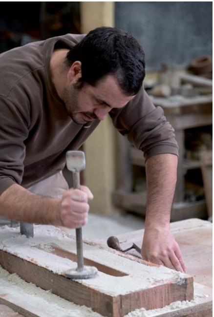
Sand casting involves constructing a mould for the bronze to be cast into: once the mould is ready and the pattern is removed, the molten bronze can be poured into the hollow area. Removing the pattern presents the most challenging aspect of the process, particularly when handling pieces with straight angles and thin walls, both essential features of this minimalist collection. Several attempts were made to hone the process, including fine-tuning specific key stages.
